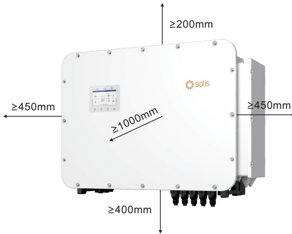
Figure 3.5 Inverter Mounting Clearances
